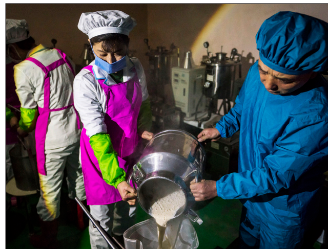
Pouring cooked soymilk through a filter press at Bongchun Children's Foodstuff Factory.
